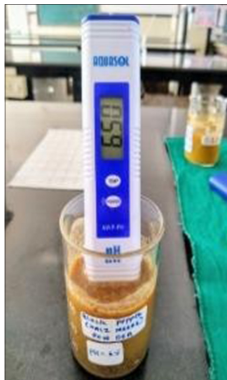
Figure 2: Measurement of pH of spices solution using a calibrated pH meter.
