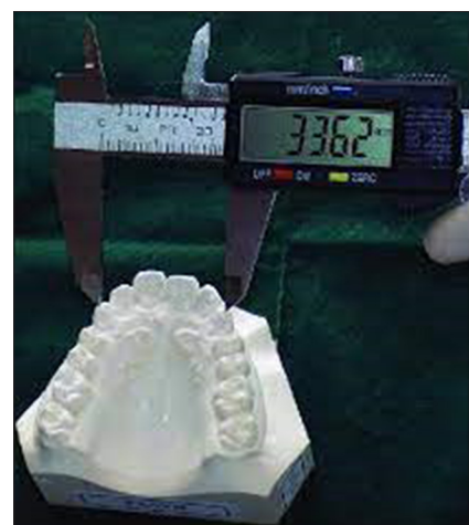
Figure 1: Pictorial representation of the intercanine distance with the Vernier calliper.
