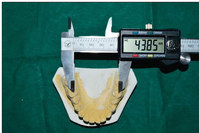
Figure 4: Measurement of intermolar arch width in mandibular study model using digital vernier caliper.
