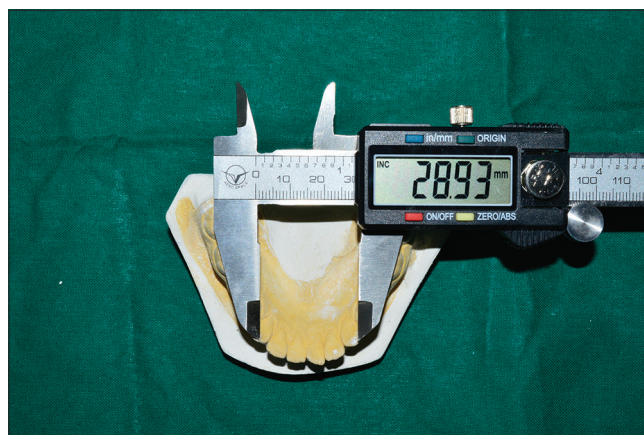
Figure 2: Measurement of intercanine arch width in mandibular study model using digital vernier caliper.
