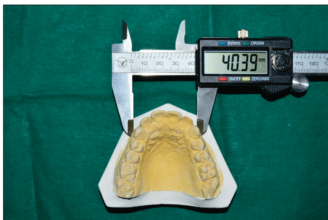
Figure 5: Measurement of canine fossa width in maxillary study model using digital vernier caliper.
